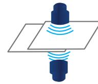
**Ultrasonic Multi-Feed Detection:** To prevent more than one document being scanned at one time the ADS-2100e uses ultrasonic multi-feed detection that ensures no documents are missed.
