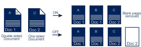
**Blank Page Detection:** When scanning a batch of documents the ADS-2100e will detect and remove any blank pages to save time and space whilst archiving.
