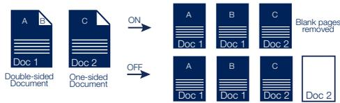
When scanning a batch of documents the ADS-1100W will detect and remove any blank pages to save time and space whilst archiving.
